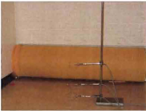
Figure 4.11 Measuring line up with anemometers at several heights and distances from the textile air diffuser
