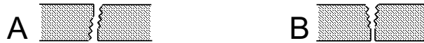
Figure 2.10: side-view of the 2 possible ways of loading the sheets into the welding machine: picture A shows the right way, picture B the wrong way.
