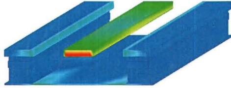
Figure 6.3: Coplanar waveguide used in the layout.
