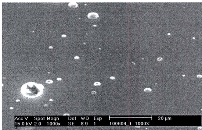
Figure 3.2 A SEM picture of sample nr.1 exposed to the debris as shown in figure3.4. The picture has a magnification of a factor 1000. The Sn-droplets, with sizes up to 10 \mu\text{m} , can be clearly seen on the surface.
