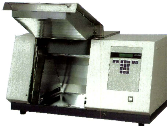
Figure 6: Photographic image of the Atlas Suntest XLS/XLS+ showing the reflective radiation chamber.
