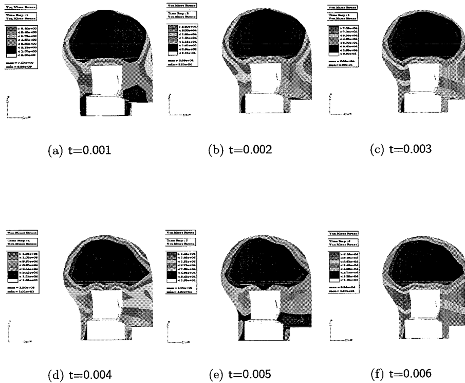
Figure B.1: Von Mises Stresses in the numerical head model
