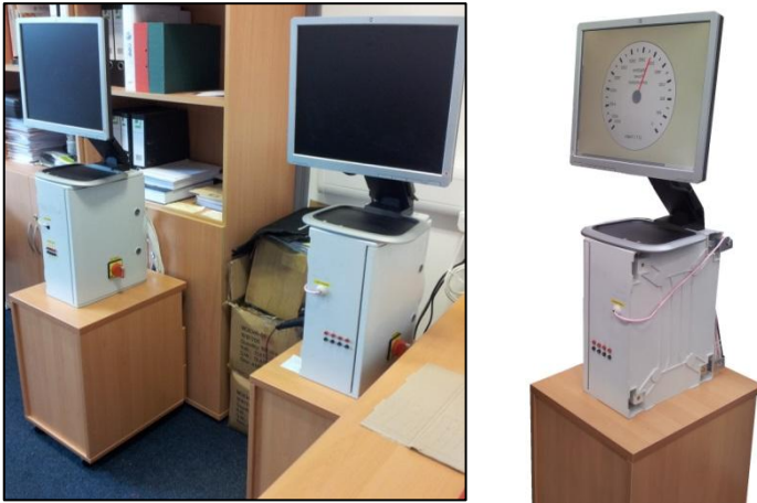
Figure 3.5. Two identical feedback devices; consisting of a screen, an encased PLC and a computer.
