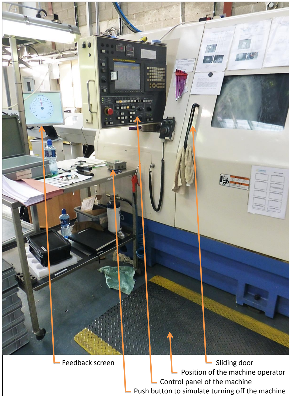
Figure 3.8. The Miyano CNC cutting machine as used in the research environment.
