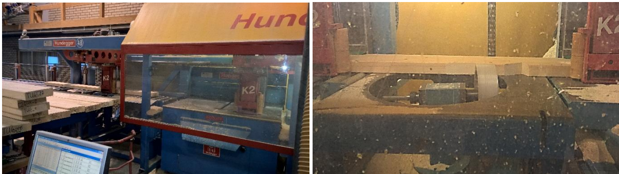
Figure 29: Specimens being fabricated with CNC cutting equipment at HEKO spanten
