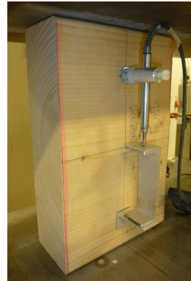
Figure 32: Compression test for perpendicular to grain loading
