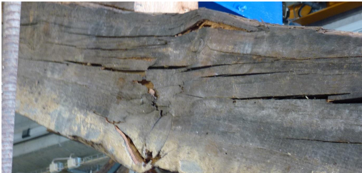
Figure 6: Small scale compression test on a Single Step Joint
