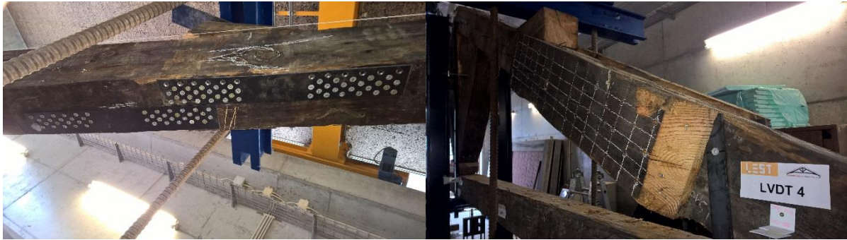
Figure 10: Left side: Mounted steel plates at the bottom.
