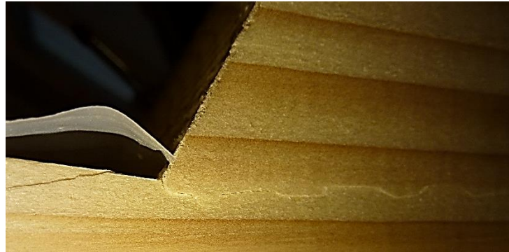
Figure 48: Visible shear cracks before the retest
