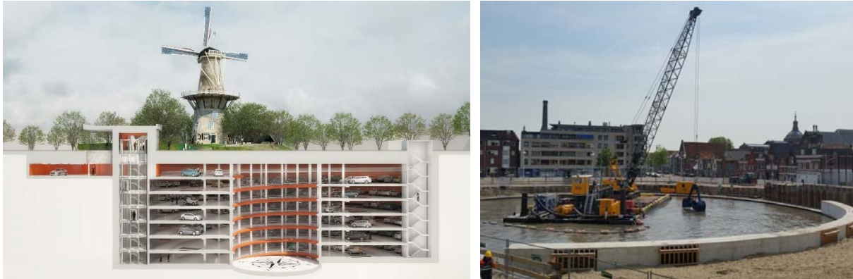
Figure A.0.3. A cross-section of the car park (left), the ground work of the subcontractor (right)
