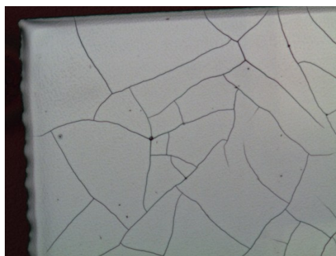
Figure 27 - Microscope image (50x) of cracks in silver
