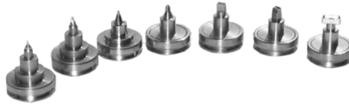
Figure 2.3: Seven different toolbit types that the AX can use. Note the different tip at the end of each toolbit.
