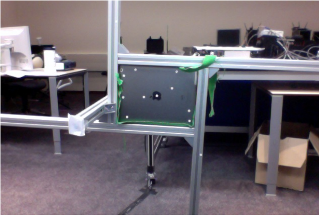
Fig. 12. 3D frame with iPad 3 attached for the experiments of Section VI-A and VI-B. Several infrared reflective markers are irregularly placed to track the orientation and position of the iPad 3.
