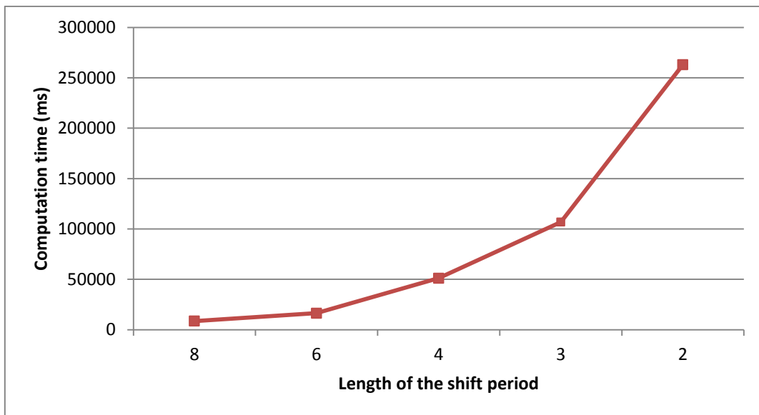
Figure 6.7: Computation time of the greedy algorithm as a function of the length of the shift period
