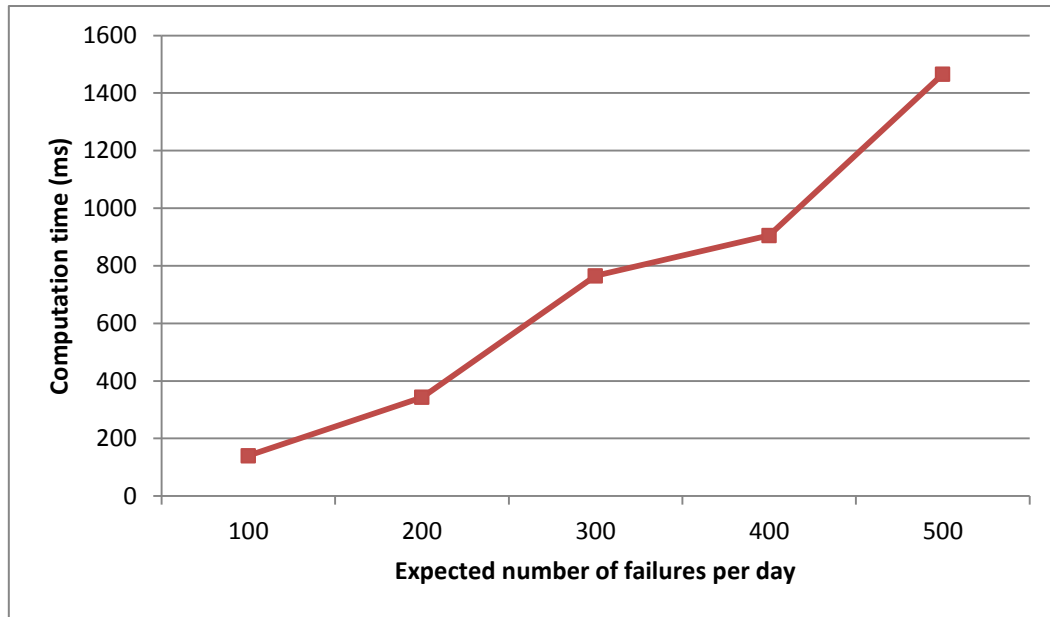
Figure 5.12: Computation time as a function of the expected number of failures generated per day. When F_{total} increases, the number of failures to be generated increases which results on the rise of the computation time
