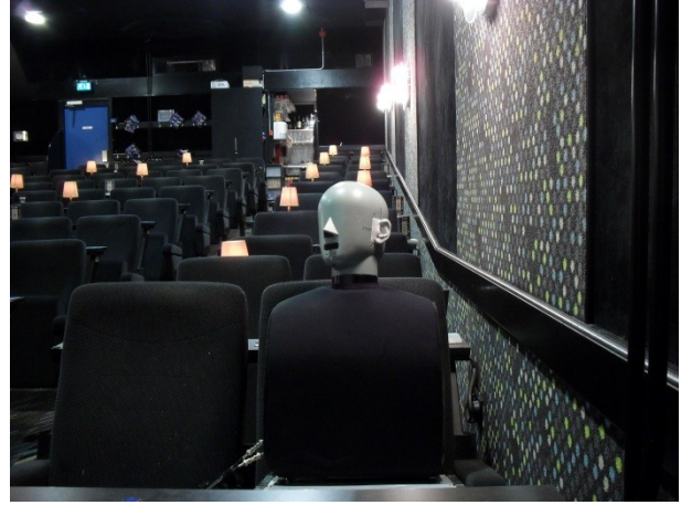
Figure 2.9 Head of HATS rotated towards screen
