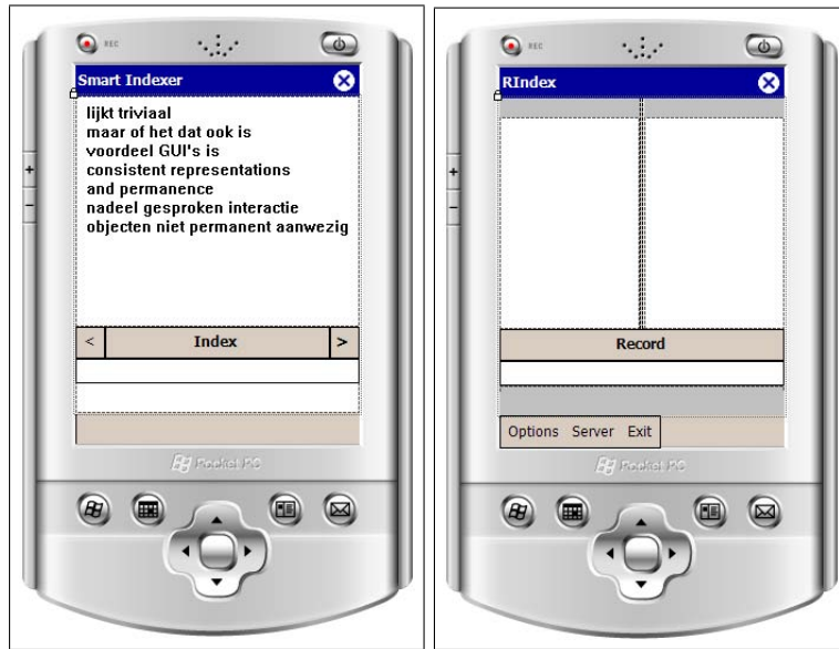
Figure 3.4: On the right side, a more refined version of the indexation interface: the list of keywords is spread over two pages, so that the user doesn't get disturbed by the system adding new keywords. On the left side (to compare), the one-page version.
