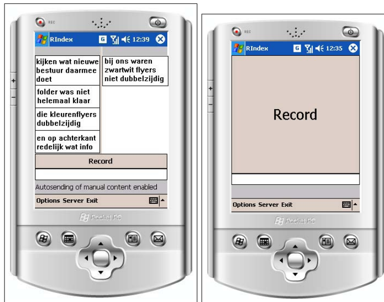
Figure 3.5: Feedback has been added to all actions (grey bar). A “simple mode” with only a “Record” button exists.
