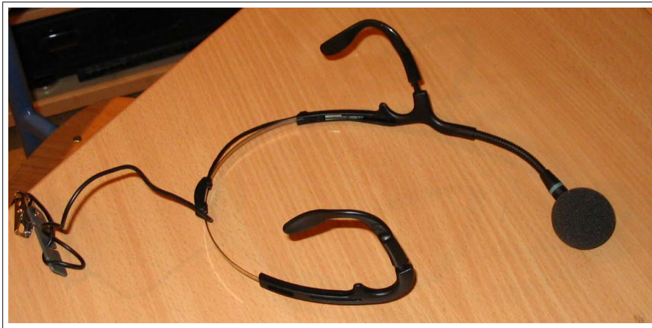
Figure C.2: The microphone: this device has a kidney-shaped sensitivity field of about 15 centimetres, which filters out the speaker's voice only and minimises the volume of the speech of others, providing a good way to separate the voices of different meeting participants.
