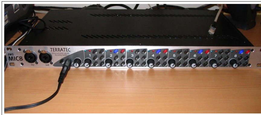
Figure C.3: The recording hardware: this Terratec sound processor can handle 8 simultaneous mono or 4 simultaneous stereo audio inputs.
