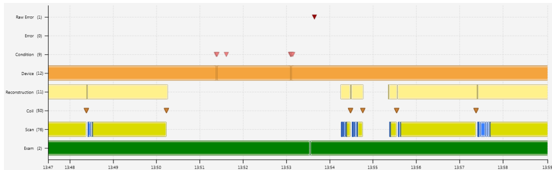
Figure 5.11: Rendering of the events using a timeline by trivially aligning the events at the time that they are produced. By looking at the events and the number of events that are supposed to be shown, it is clear that the glyphs are overlapping. The coil category should show 50 glyphs, but only 6 are shown. The events in the device and the coil category seem to suffer the most from this.
