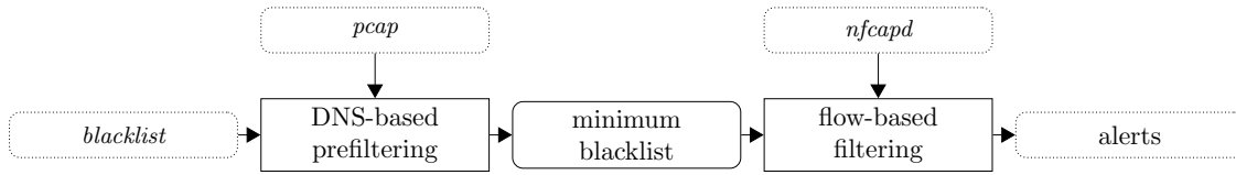
Figure 5.1: Approach for Scenario 1 and Scenario 2 using DNS-based prefiltering before performing flow-based filtering. The rectangles are processes. The rectangles with rounded corners are data and, specifically, the dotted are input or output of the system.
