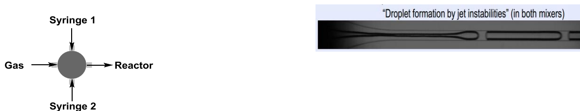
Figure 4: Schematic view of a cross mixer and the Taylor flow created in the cross mixer
