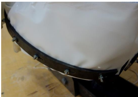
Figure 81: Clamping of outer fabric layer
