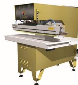
Figure 4: High frequency welding (Forsstrom, N.D.)
