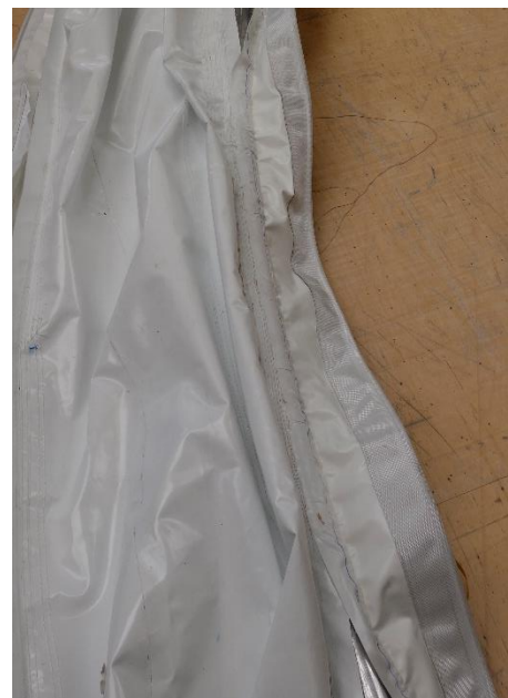
Figure 71: welding the outer layer
