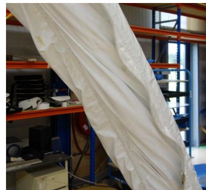
Figure 77: Wrinkles in the fabric prior to heightening the compression elements
