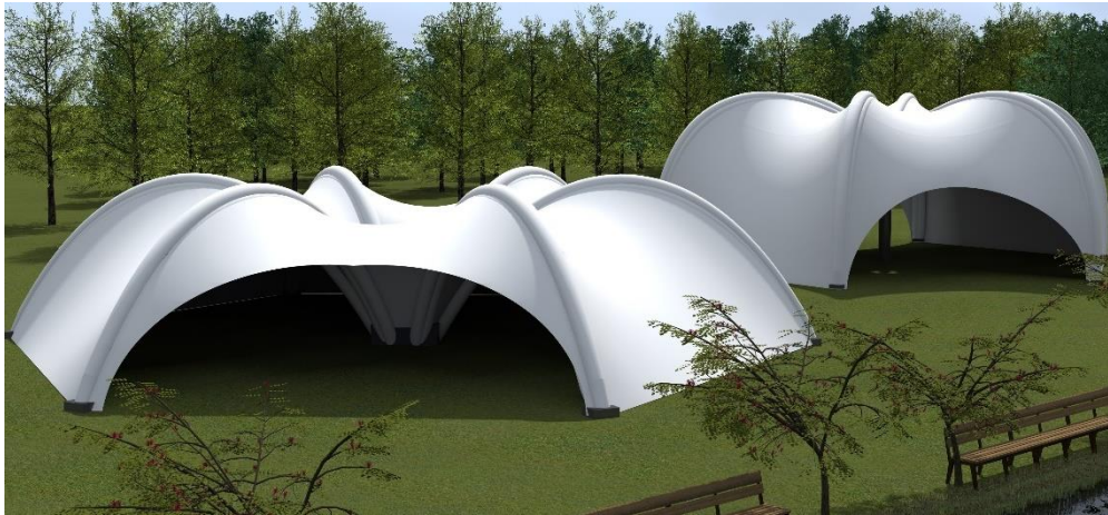
Figure 21: Second alternative design (left: arches join at bottom, right: arches join at top)
