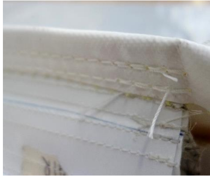
Figure 67: Closing seam of web onto sleeve (Figure 65, blue line)
