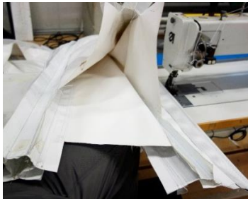
Figure 69: Fabric web closed, overview (Figure 65, red and blue line finished)
