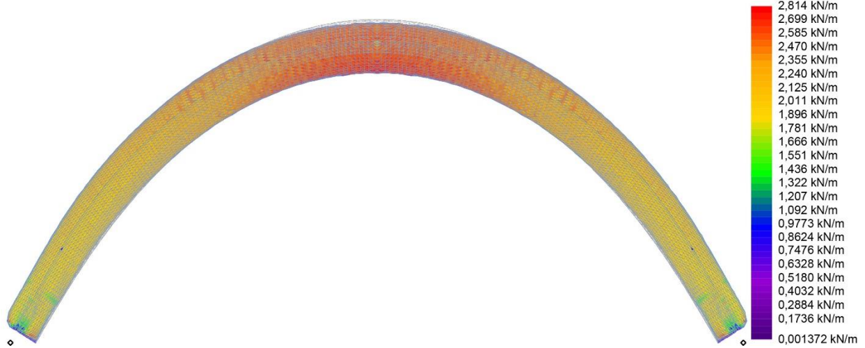
Simulation results with a load distributed over five points (2D-force Nx, deformation magn. x8)
