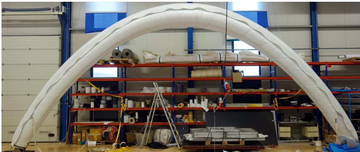
Figure 86: Construction of tensairity arch completed
