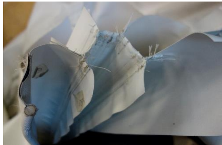
Figure 70: flat seam between outer layer and sleeve (Figure 65, green and pink line)
