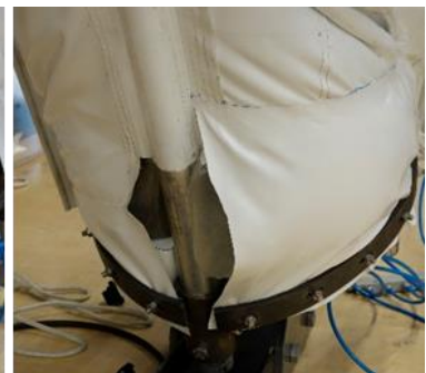
Figure 80: left; without additional fabric, right; with additional fabric
