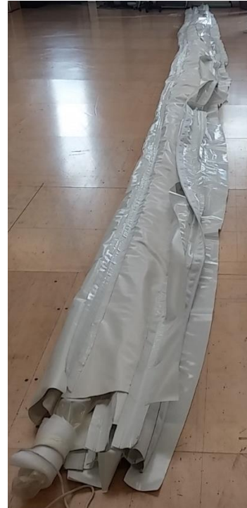
Figure 68: Stitching of fabric hull finished
