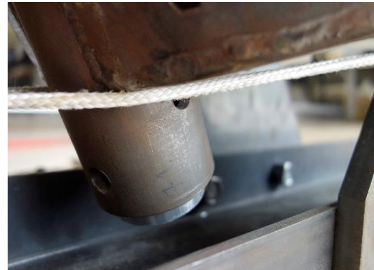
Figure 75: Imposition retracted too little
