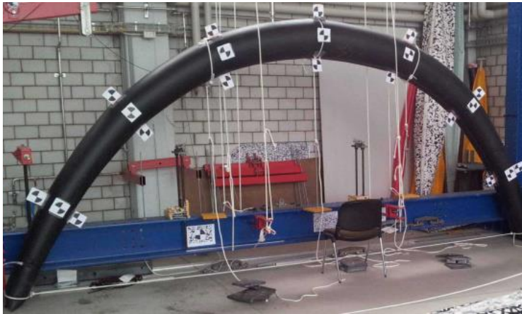
Figure 108: Tensairity arch of R. Maffei
