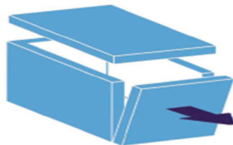
Figure 5-2 Out of plane wall failure
