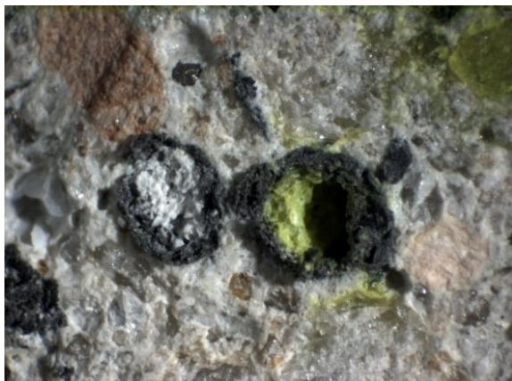
Figure 23: Two PCM particles from whitch one is broken.
