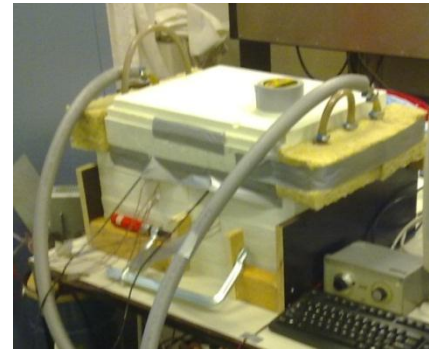
Figure 45: setup with the taped up cracks
