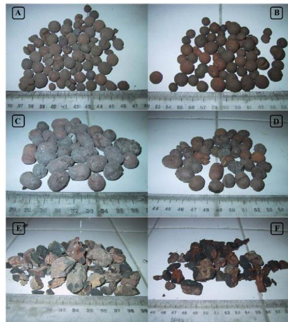
Figure 11: Unfilled(left) and filled(right) lightweight aggregates
