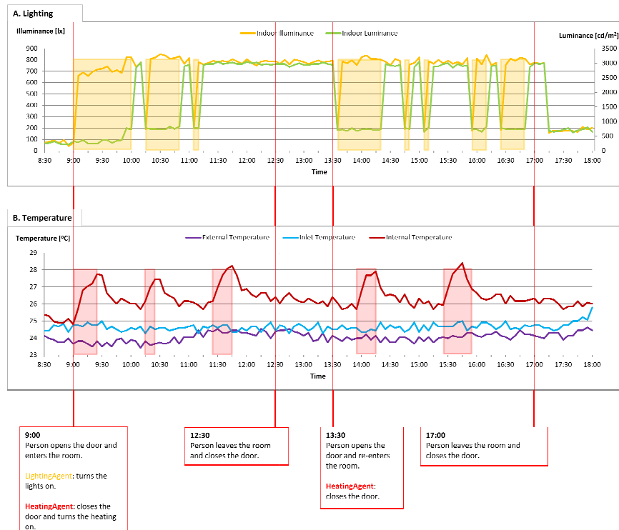
Figure E-11a: The same as figure E-11, except this time the lighting and heating loads are included in the graphs.
