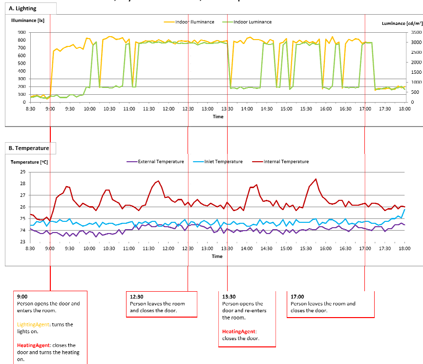
Figure E-11: Results of energy saver with MAS control and dynamic blinds. This scenario represents a regular working day in winter. The person working in the room is someone who tries to save energy whenever possible. The person enters the room at 9:00, sets the thermostat to 26 °C and leaves for home at 17:00. Between these hours he never has to turn the heating or lighting on or off and never has to raise or lower the blinds, because he can fully rely on the MAS for the control of all these three systems.
