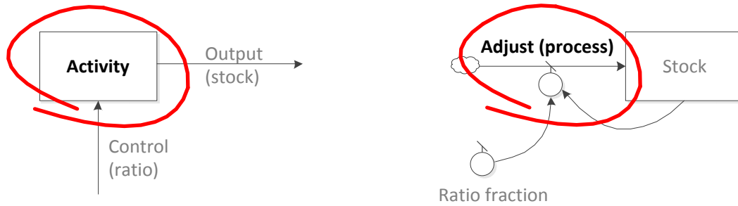
Figure 5.7 SADT activity boxes (l) are translated to stock and flow diagrams (r) of SD (source: Hommel & McGowan, 1989)
