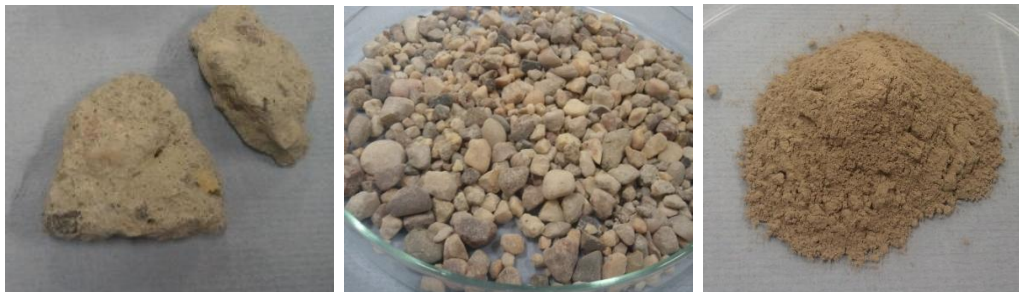
Figure 4.3 Concrete after pre-crushing (left), recycled concrete gravel and sand (middle) and recycled concrete fines (right)
