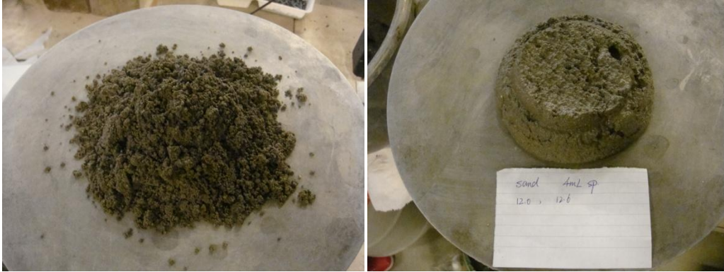
Figure 4.26 RCS mortar samples without SP (left) and with SP (right)
