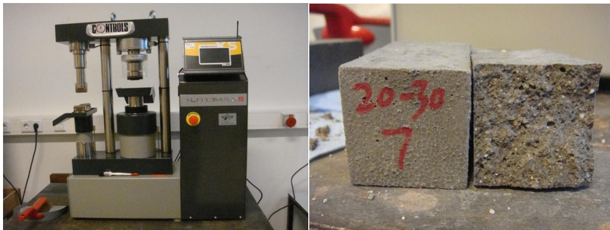
Figure 3.10 Mortar strength test machine (left) and fractured mortar sample (right)
