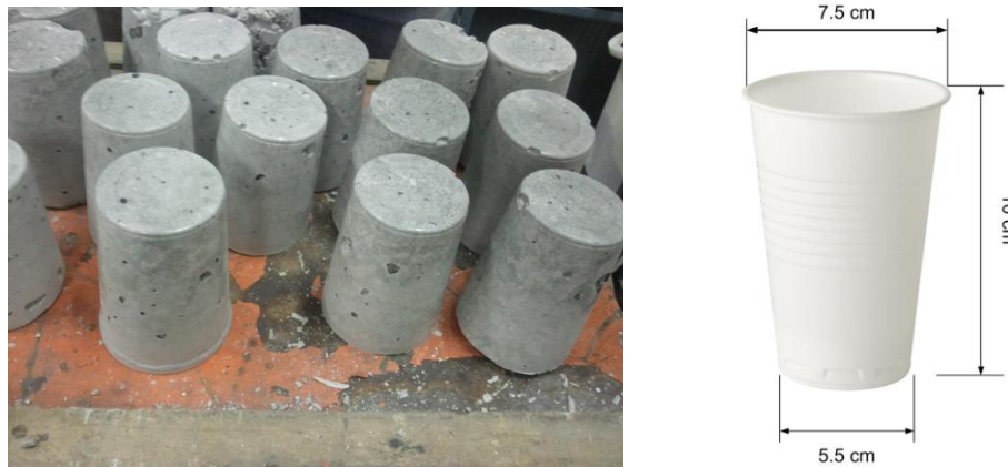
Figure 4.2 Cup concrete and the dimension of the plastic cup
