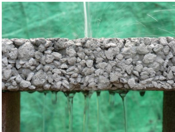
Figure 2.7 Pervious concrete pavement
