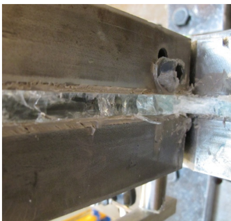
Figure 4.26 Close up adhesive joint RTC. (HSG 1 after glass pane failure)
