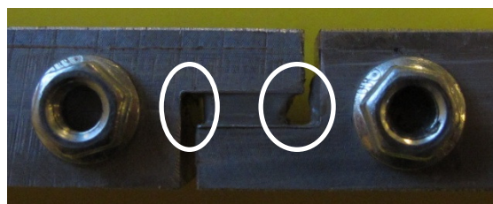
Figure A.6 Bonded joint with less bonding area.
