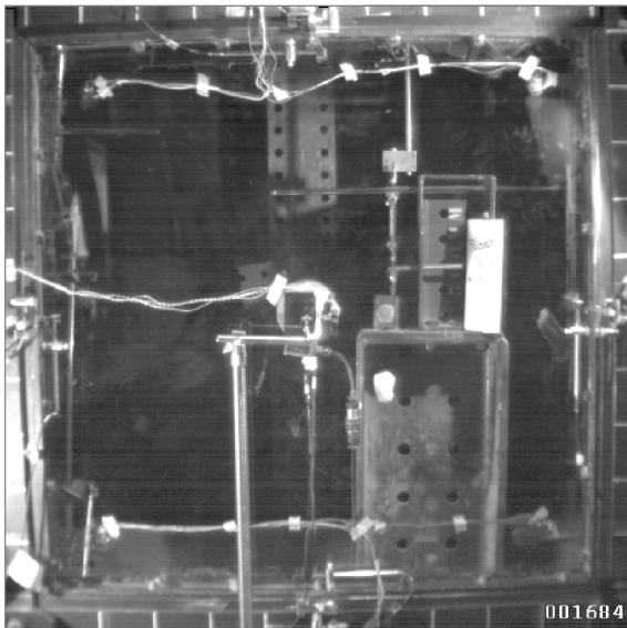
Figure 4.37 (left) Un-cracked glass pane one four thousand of a second before moment of fracture.
