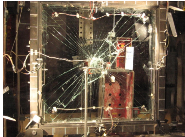
Figure 4.31 Cracked glass pane.
