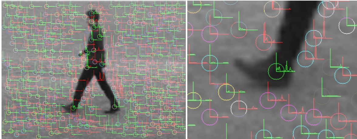
Figure 21: Local descriptors as orientation histograms of the magnitude. Green histograms are bottom-peak-critical-points, red histograms are top-peak-critical-points.
