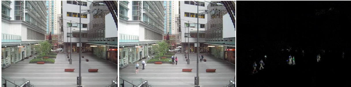
Figure 1: Background segmentation steps. From top left to top right: a) background image, b) video input, c) background subtraction.
