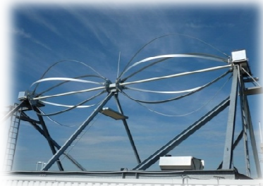
Figure 2.4 – HAWT with a fastened axis “WindWall” (Cace et al., 2007)
