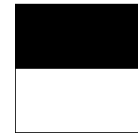
Figure 4.13: Haar wavelet filter to compute response in y-direction, image from [BETVG08]
