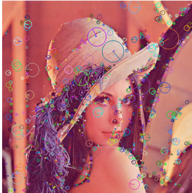
Figure 8.3: Keypoints detected using GPU SIFT. Circle size denoted the size, the line denotes the orientation.
