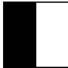
Figure 4.12: Haar wavelet filter to compute response in x-direction, image from [BETVG08]
