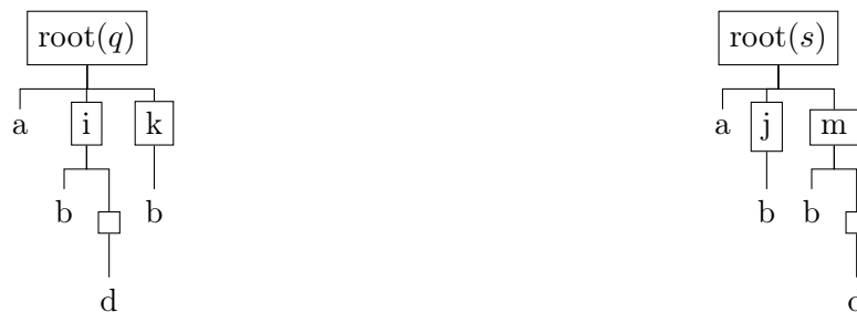
Figure 4.10: An example of an iso- and homomorphic containment, i.e., the left tree, query q , is contained in the right tree s .
