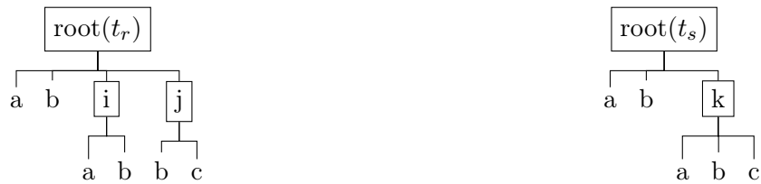
Figure 3.1: The tree representation of the nested sets relations t_r and t_s . Note that identifiers are used to identify leaf values and children, e.g., \text{nodes}(\text{root}(t_r)) = \{i, j\} , \text{leaves}(\text{root}(t_r)) = \{a, b\} and \text{leaves}(k) = \{a, b, c\} .
