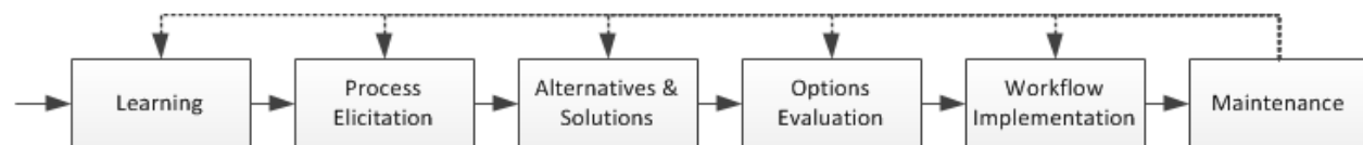
Figure 2 – The PAWS approach [9] with six consecutive phases; the dotted line indicates paths taken during the maintenance phase. The maintenance phase can be considered as a 'mini reengineering cycle'.
