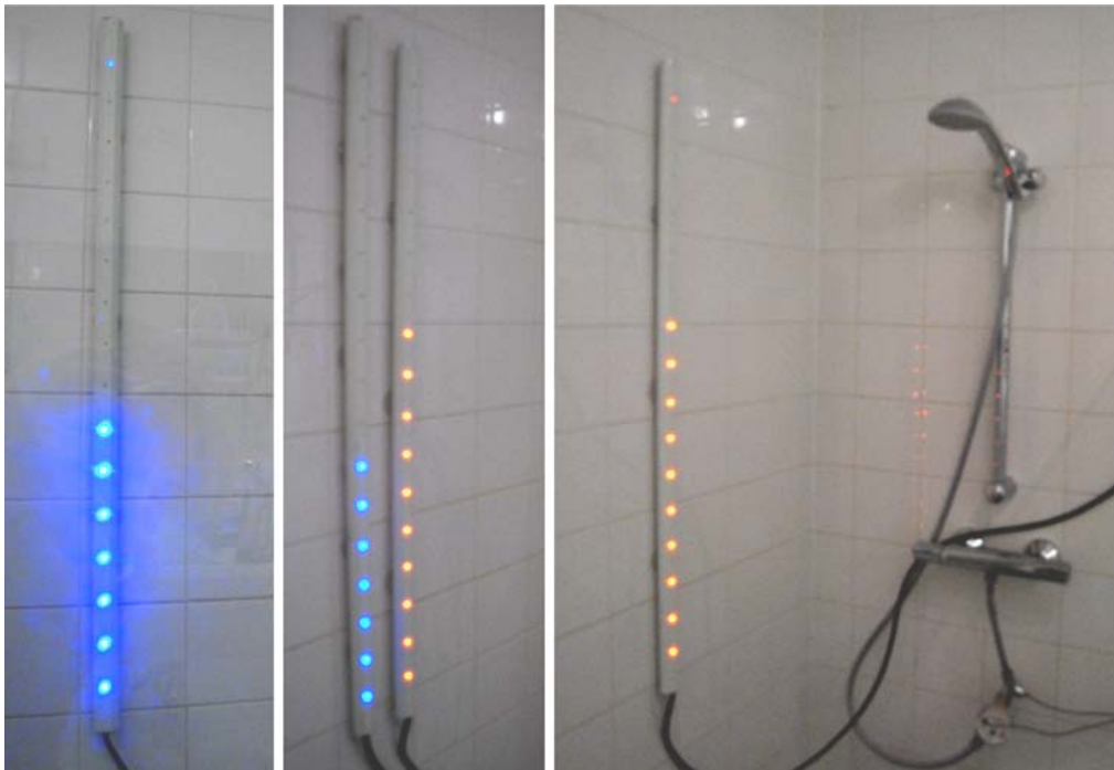
Figure 2. Shower meters installed in the shower. From left to right: water feedback, water & energy feedback, energy feedback.
