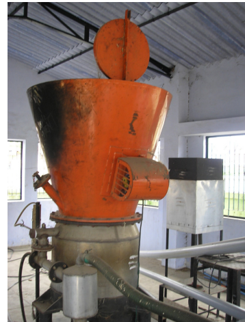
Fig. 4.12: A 9 kW Ankur gasifier reactor
