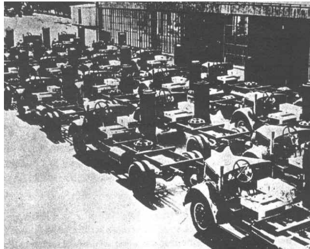
Fig 4.1: A mass production line of biomass gasifier cars in Germany in 1943 (Source: Biomass Energy Foundation)
