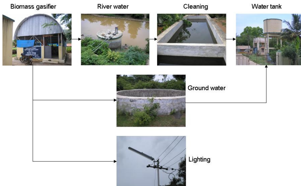
Fig. 5.11: The applications of the biomass gasifiers
