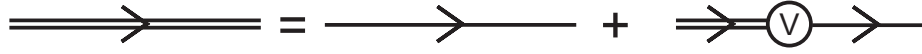
Figure 5.3: The Dyson equation 5.6 in Feynman diagrams. The double lines represent the propagators for electrons in the interacting system, the single lines represent the non-interacting electron propagators and the circle V represents the electron self energy, which contains all the interactions. A similar diagram can be drawn to visualize Dyson equation 5.7
