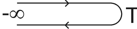
Figure 5.2: The Keldysh contour is the timeline in which time goes from -\infty to time T and back to -\infty , where eventually T \rightarrow \infty .
