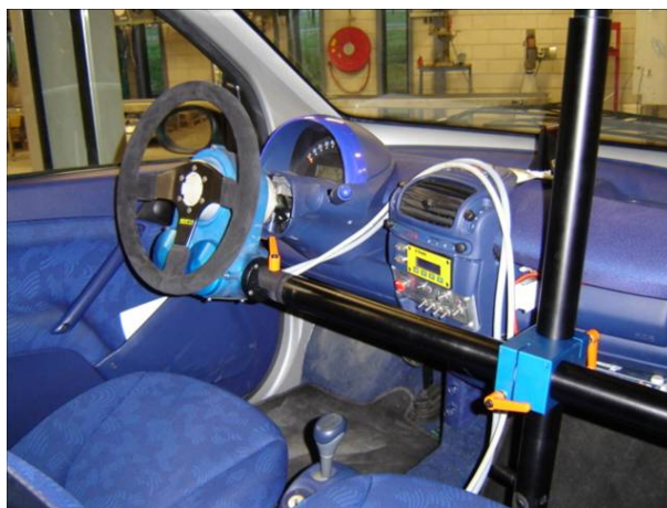
Figure 2.2: Steering robot installed in Smart
