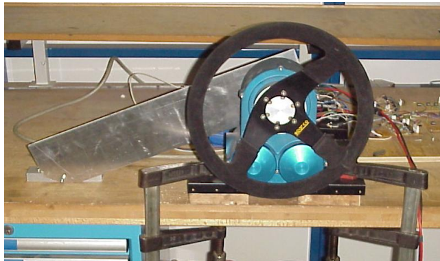
Figure 6.3: The locked steering robot
