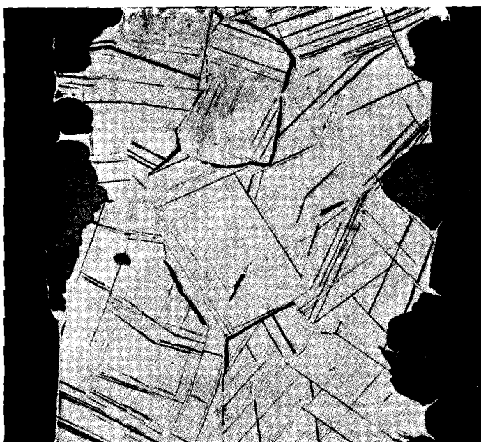
Fig. 10. Metallographic cross-section of tantalum specimen oxidized for 3900 min at 1500^{\circ}\text{C} and 10^{-4} torr \text{O}_2 . ( \times 100 )
