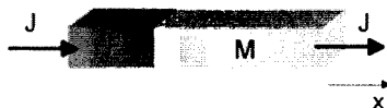
Figure 2.7: Schematic representation of the experimental layout for which the Boltzmann equation will be solved. A current J is flowing through a ferromagnetic-nonmagnetic system.
