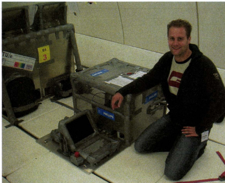
Figure 5.4: The Parabolamp experiment mounted in the zero-g airplane. To the left of the Parabolamp experiment, the ARGES measurement setup is visible.
