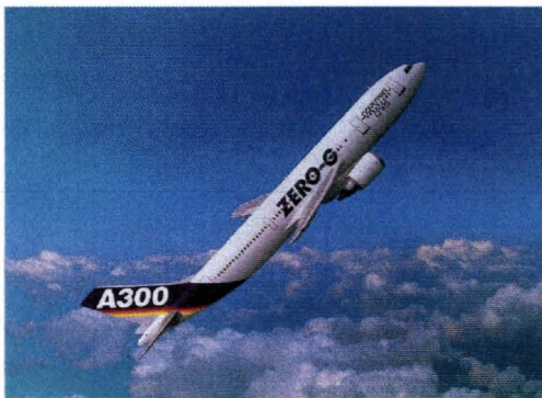
Figure 1.3: The zero-g airplane at the injection point is shown on the left picture. Details of a single parabola including a rough timescale can be seen in the drawing on the right.
