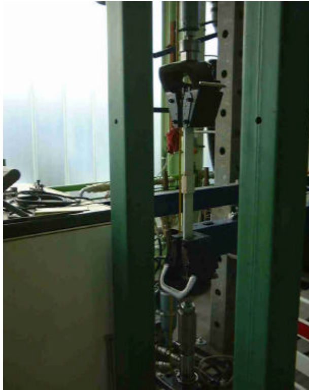
Figure 25: experimental set-up for the double lap joint
