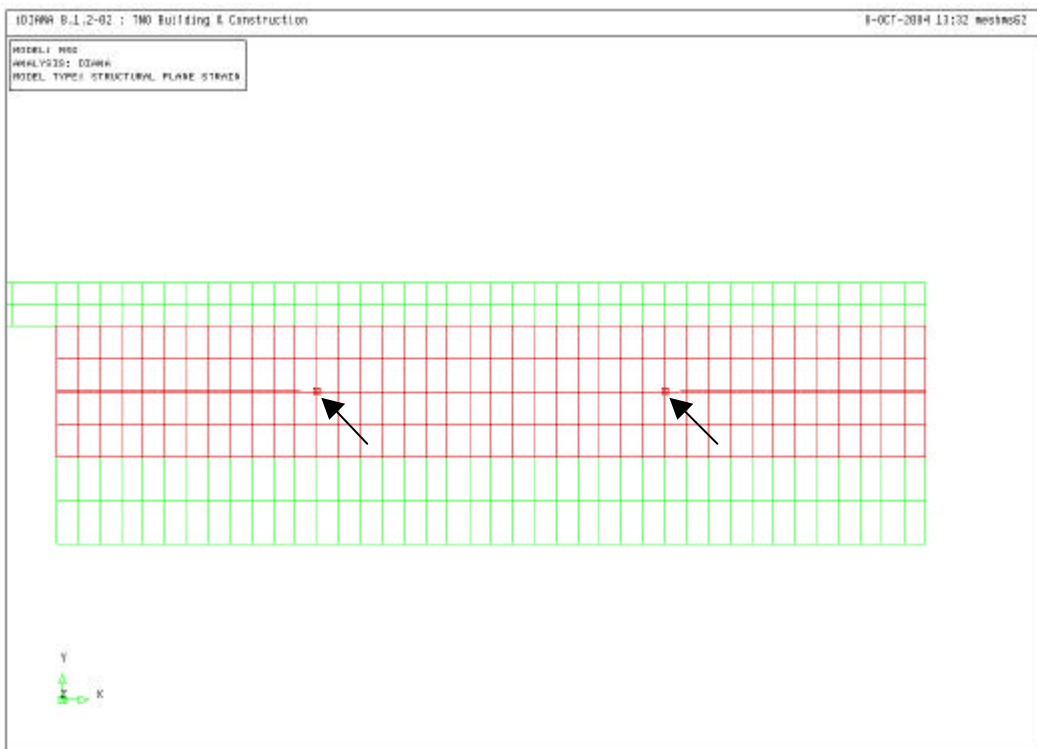
Figure 38: mesh in the adhesive layer around the crack tip (MS polymer)
