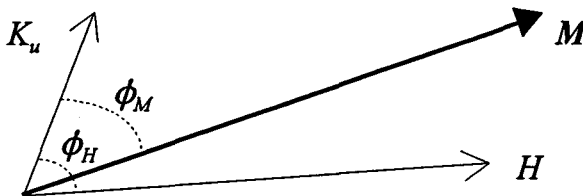
Fig. 2.4 Rotation of magnetization in a single domain.
