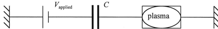
Figure 4.24: A capacitor can be connected in series with the plasma in order to represent the liquid crystal layer.
