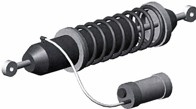
Figure 5.11: Coil-over spring-damper with oil reservoir
