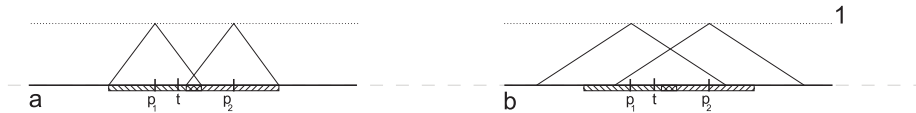
Figure 3.6: Two point samples p_1 and p_2 are shown. The two radii are indicated with a different hatching. An arbitrary texel t that falls within the domain is also shown. In a , the basis function width is chosen as large as the point's radius. In this case this means that f(t) < 1 . In b it is chosen larger, so that f(t) \geq 1 . However, the basis functions now extend over the domain's border. This causes the domain primitive to represent the domain as if it were larger than it in fact is.
