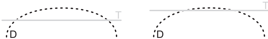
Figure 3.1: The plane T resulting from non-weighted PCA on the points in domain D is shown on the left. The result of weighted PCA is shown on the right.
