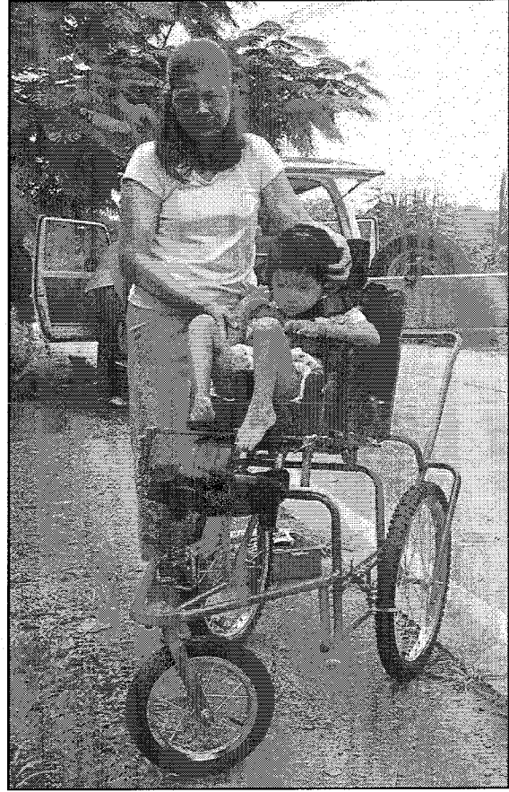
Figure 29. Bantitaa enjoys riding in her CP-buggy. Although the seat is very comfortable, the footrests are a point of improvement. The height of the seat is a concern of many caregivers and makes it difficult to interact with other children.
