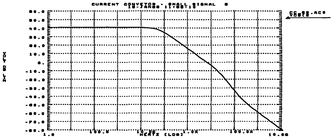
Figure 4.9: The open-loop gain (magnitude) of the current-conveyor.
