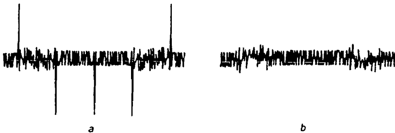
Figure 3.14: Typical Kasami code family a) ACF b) CCF over a period of 5 sequences.
