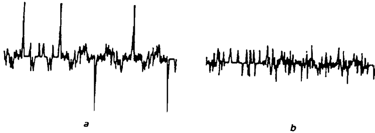
Figure 3.12: Typical Gold code family a) ACF b) CCF over a period of 5 sequences.
