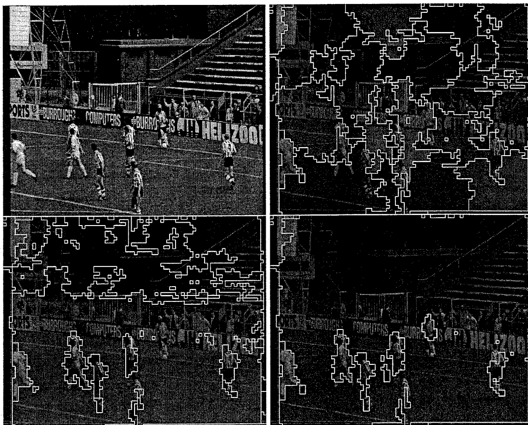
Figure 5.6: K -models clustering of frame 21 of the football sequence with K=16 . Edges between clusters are denoted with a white line. Top right picture is generated with a 2 parameter affine model, the bottom left picture with a 4 parameter affine model and the bottom right picture with a 6 parameter affine model. It is clearly visible that the 2 parameter affine model suffers from the camera zoom in this sequence.
