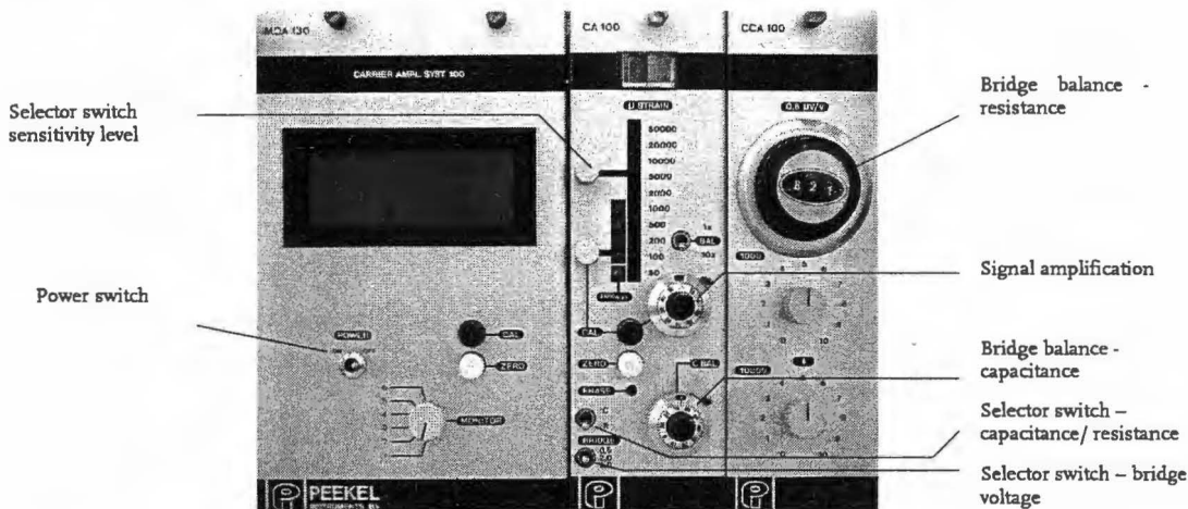
Figure I.1: Peekel Instruments Carrier Signal Amplifier with MCA130, CA100 and CCA100 components
