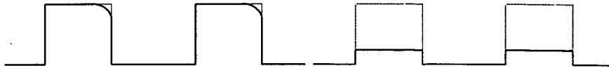
Figure 4: Schematic representation of the process effects. The left picture shows the asymmetric corner rounding, while the right picture shows the alteration in optical depth.
