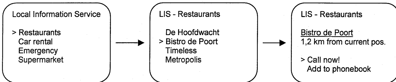
Figure 7. Example of the Location Information Service. The user selects the link indicated with ">".
