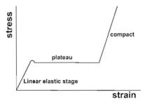
Figure B.3: Typical stress-strain relationship for foam materials in compression.
