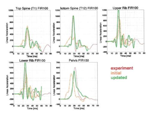
Figure E.7: Results for EBS 00/100/00-without-jacket test
