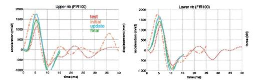
Figure 4.2: Results for thorax component test (v = 8.3 m/s). Test results vs. initial, updated and final predictions.
