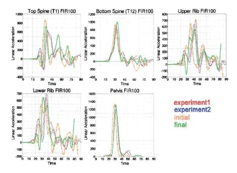
Figure 6.8: Results for 00/150/100 EBS test
