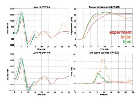
Figure E.2: Results for thorax component test (v = 8.3 m/s).
