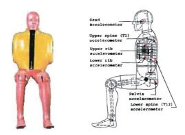
Figure 2.1: The US-DoT Side Impact Dummy.
