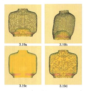
Figure 3.19: Build-up of the jacket geometry. a) and b) the outer jacket in wireframe, the shelf in solid yellow and the brigde in solid orange c) Jacket mesh in single layer ISOLIN shells d) Jacket mesh in dual layered shells (one ISOLIN and one ISOTEN).
