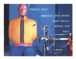
Figure 4.4: DoTSID crash test dummy in an abdomen leading linear guided impactor test set-up.
