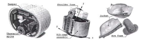
Figure 2.6: The US-DoTSID upper torso, containing the thoracic spine and rib cage assembly (left and middle) and the jacket and arm foam (right).
