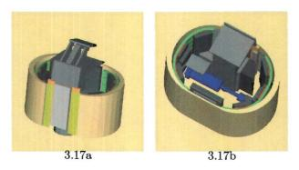
Figure 3.17: Connecting a) the thoracic spine assembly and b) the damper unit.
