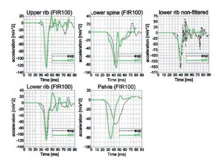
Figure 5.6: Results for GM-SUV FMVSS201 impact.
