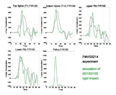
Figure 6.2: Comparisson of the GM-FMVSS214 experiment (black) with the 00/150/00 rigid impactor model prediction (green).
