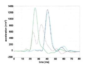
Figure 6.6: A comparisson of the predicted pelvis accelerations (g) for the 00/150/100-3cm-up simulation (green), the 00/150/100-3cm-up (red) experimental results and the experimental results from the 00/150/100 test (blues).
