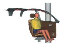
Figure 5.5: Analysis of GM-SUV FMVSS201 pole impact.
