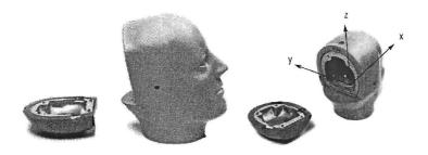
Figure 2.11: The US-DoTSID head.
