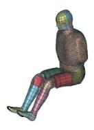
Figure 1.7: FAT finite element model of the US-DoTSID.
