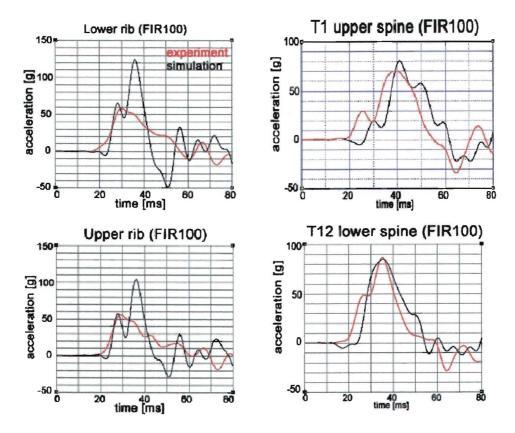
Figure 5.2: Analysis of GM-vehicle FMVSS214 impact. Red lines denote the experiment, black lines denote the predicted values.
