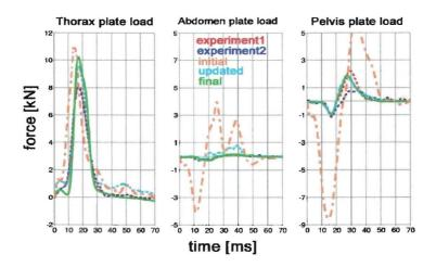
Figure 4.6: Impactor plate loads for the 50/00/00 stagered impact test
