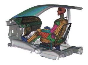
Figure 1.6: Example of FE and facet model combination.
