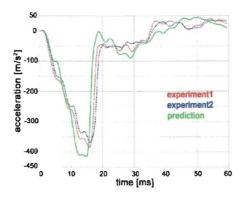
Figure 4.3: Predicted (green) vs experimental (blue and red) impactor acceleration for the pelvis component test.
