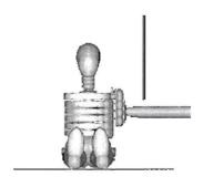
Figure 1.4: Multibody model of the SID-IIS dummy.
