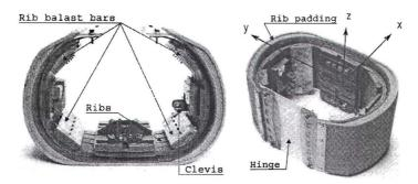
Figure 2.8: The US-DoTSID rib cage assembly.
