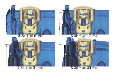
Figure 5.3: Analysis of GM-vehicle FMVSS214 impact.
