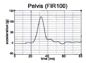
Figure 5.4: Prediction of pelvis acceleration in GM-vehicle FMVSS214 impact.
