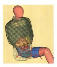
Figure 3.1: Hybrid multibody-FE DoTSID.
