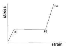
Figure B.4: Three point representation of a typical foam loading curve.
