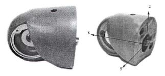
Figure 2.13: The US-DoTSID post knee assembly.
