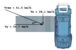
Figure 5.1: Test set-up for FMVSS201 procedure.
