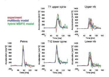
Figure 4.9: Results for 00/50/50 deforming barrier test. A comparison between the predictions of the hybrid MB/FE DOTSID model and the multibody model with respect to the experimental values.
