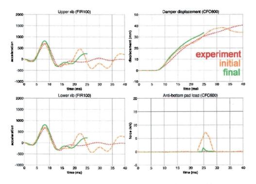
Figure E.1: Results for thorax component test (v = 4.1 m/s).
