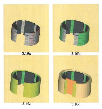
Figure 3.16: Build up of the ribcage assembly with a) the rib steel strips, rib ballast bars and dampening cushions. b) Rib damping material. c) Rib wrap and d) Rib padding and hinge.
