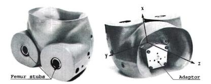
Figure 2.3: The US-DoTSID lower torso.
