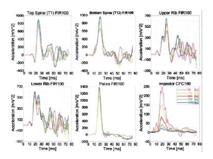
Figure 6.1: Mass sensitivity study for the 00/150/100 rigid impactor.
